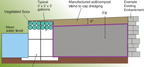
Additional aggregate to create a base for the gabion above the substrate
