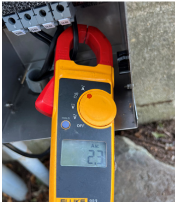
4b. Secondary Amperage reading at first fixture or connection; CORRECT WAY
